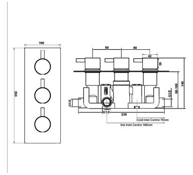
Dimensions are in millimetres except thread sizes which are BSP imperial.
