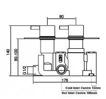
Dimensions are in millimetres except thread sizes which are BSP imperial.
