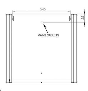
\*Dimensions are subject to change, customers are advised to measure actual product before commencing installation. \*\*Fixing point dimensions are for guidance only/the positions of wall fixing must be checked when product is received.
