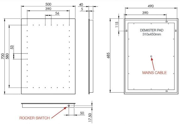
\*Dimensions are subject to change, customers are advised to measure actual product before commencing installation. \*\*Fixing point dimensions are for guidance only/the positions of wall fixing must be checked when product is received.
