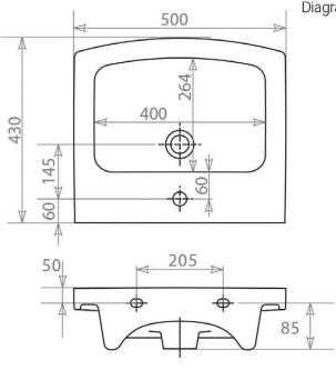
Diagrams not to scale. All dimensions in mm (tolerance of +/-5mn  $\,$
